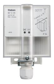
Radio control via antenna with top2 RC devices: To ensure good reception, do not install the antenna in cellars or on distribution boxes. Connection is made via separate 2-wire, unscreened high-voltage power cable (max. 100 m), up to 10 Theben top2 RC devices can be connected. Polarity, short-circuit and interruption of the antenna circuit are each visually displayed to help with installation.
